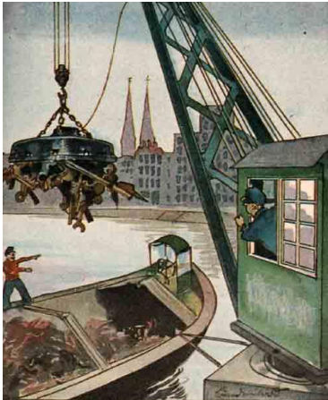
Figure 1 Loading of metal waste with a large electromagnet
